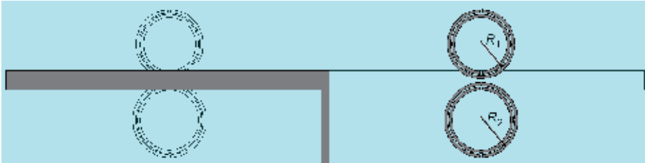
Fig. 11. Sketch of the proposed triple-frequency printed dipole loaded with SRRs.
