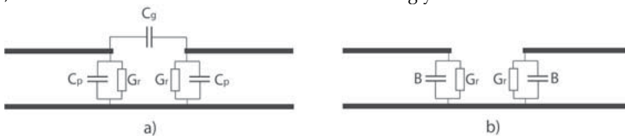
Fig. 13. a) Theoretical equivalent circuit model of inner slot R-EAN, b) implemented admittance network
