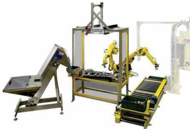
Fig. 1. Vision Guided Robotic Flexible Feeding (Christe, 2009)
