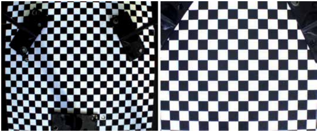
Fig. 3. The chess-board pattern seen by the Point Grey camera with a 4mm (left) and a 6mm (right) lenses respectively.
