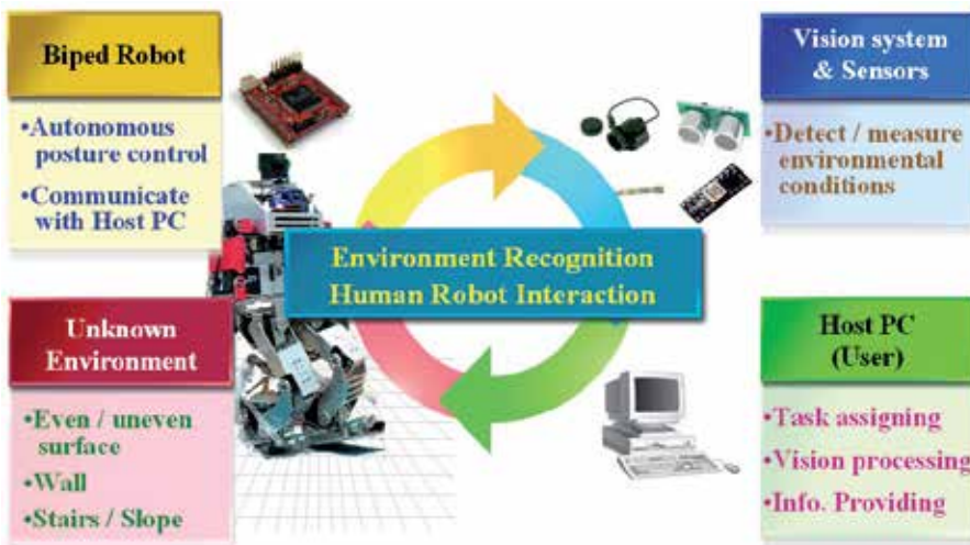
Fig. 1. Overall system architecture
