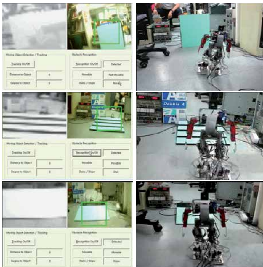
Fig. 15. Obstacle Recognition Results for a wall(top), stairs(middle), a slope(bottom)
