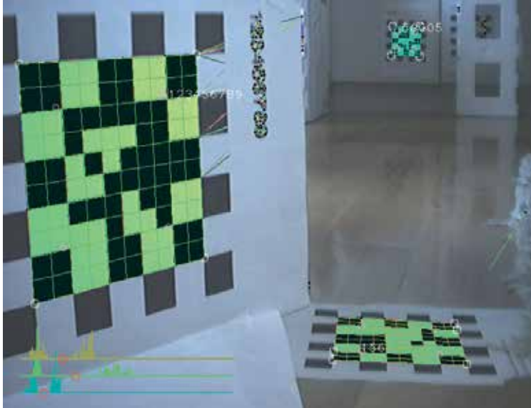
Fig. 3. Three landmarks visible in the same scene to demonstrate the limitations. All landmarks have a frame width of 17.5cm. The near is at 0.46m and the far at 3.2m, the one on the floor is tilted 79^\circ . The image resolution is 640 \times 480 pixels.
