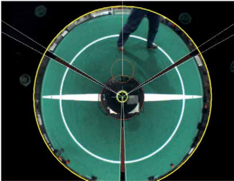
Fig. 10. Automatic extraction of main image features, while robot is standing at the center of a MSL middle field circle.
