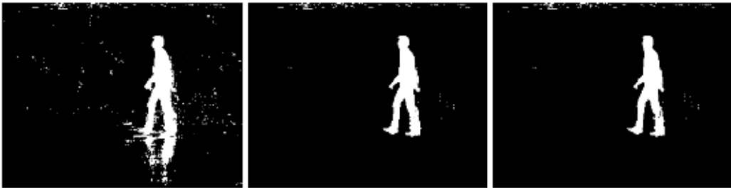
Fig. 16. Three segmentation results with varying values of \sigma . Left: \sigma -value too low. Middle: optimal \sigma -value. Right: \sigma -value too high.
