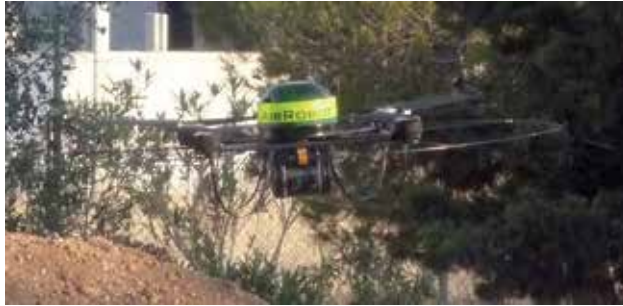
Fig. 4. The AR-100 UAV with the camera mounted beneath the flight board.
