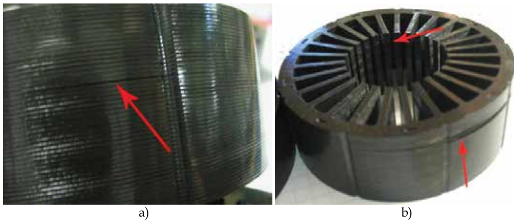
Fig. 9. Slots inside and outside (a, b) and broken EM stator (b)
