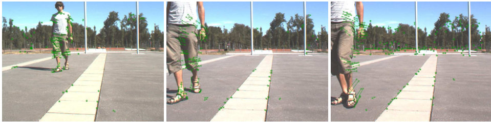
(a) Input images for the obstacle detection: the black star is the epipole and the green vectors are the optical flow.
