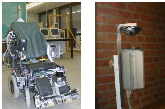
Fig. 1. Left: the robotic wheelchair platform. Right: the omnidirectional camera, composed by a colour camera and an hyperbolic mirror.
