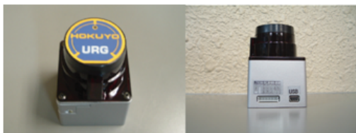
(a) External appearance Fig. 8. Laser range scanner, URG-X002
