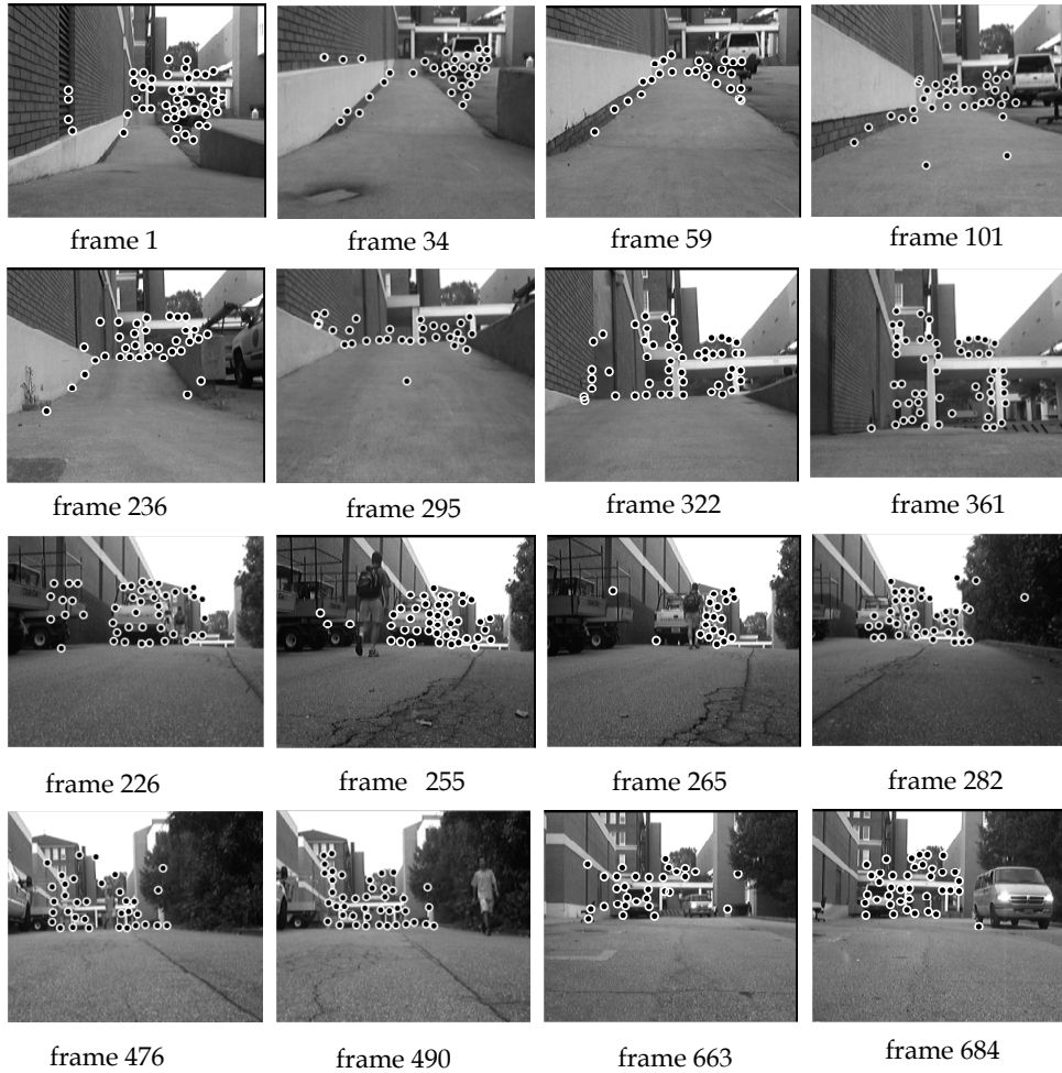
Fig. 10. Sample image frames from two different sequences, one in which the robot traveled down and up a ramp (top 2 rows), and the other containing dynamic objects (bottom 2 rows). The circles indicate the features.
