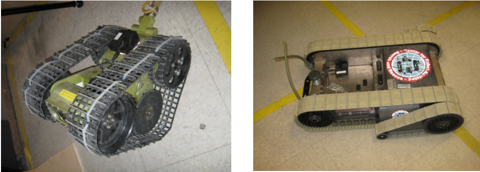
Fig. 1. The Inuktun MicroVGTV and I-Robot Packbot was used in the rescue attempts at the World Trade Center in September 2001
