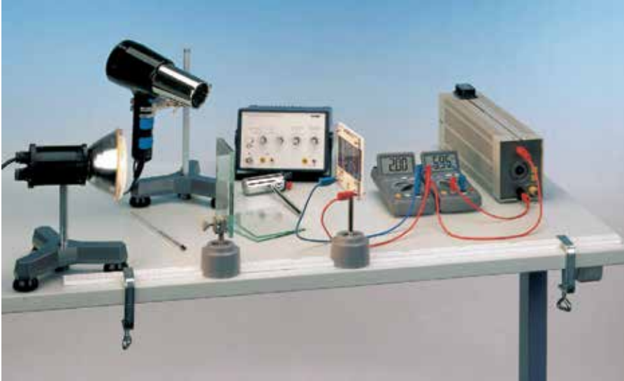
Fig. 4. Experimental set-up of silicon solar cell illuminated with a direct light from a lamp.
