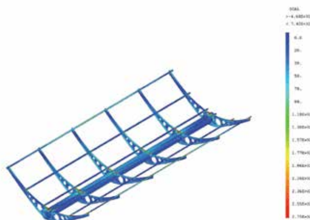
Fig. 11. Contour map of maximum equivalent Tresca stresses for w3p060c1.
