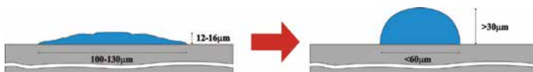
Fig. 16. Future improvement of the metal finger cross-section
