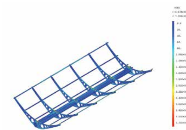
Fig. 12. Contour map of maximum equivalent Tresca stresses for w4m120c9.
