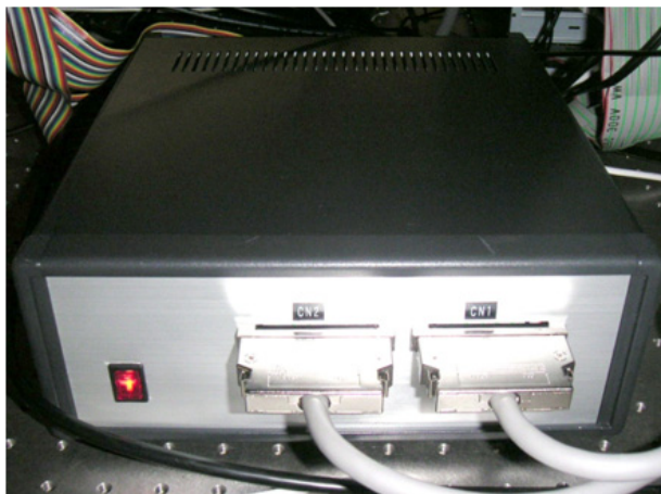
Fig. 7. Electrical part of the compact laser communication transceiver
