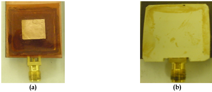
Fig. 22. Optical images of the assembled stacked antennas (a) microstrip fed and (b) CPW fed device.
