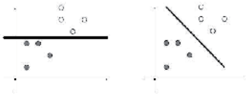
Fig. 7. A separator that the margin is not maximized, have less good generalization properties than that which the margin is maximized.
