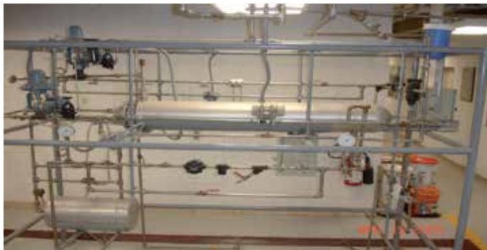
Fig. 17. Industrial heat exchanger used in the experiments.
