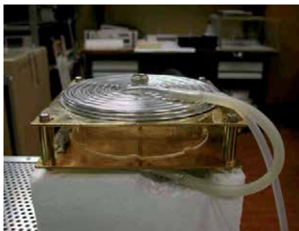
Fig. 19. Exaple of WPC with cooling system as two water spiral-plate jackets placed on external faces of WPC.
