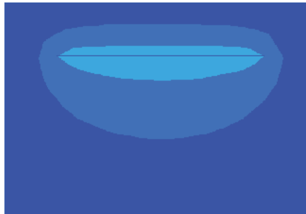
Fig. 8. Temperature distribution due to E field below the septum from fig.7. Temperature in the middle 15cm below septum is 300.003 K ( E=3.28\text{V/m} )
