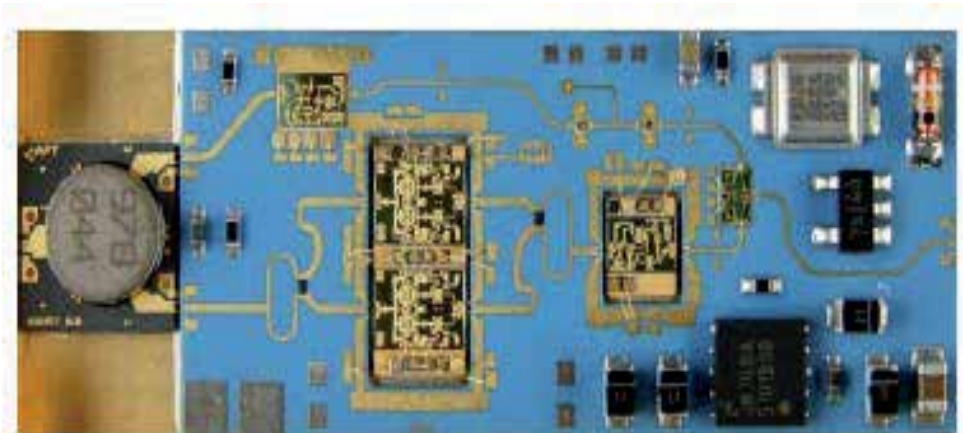
Fig. 2. Photo of a T/R-Module front-end with GaN MMIC chips [31]
