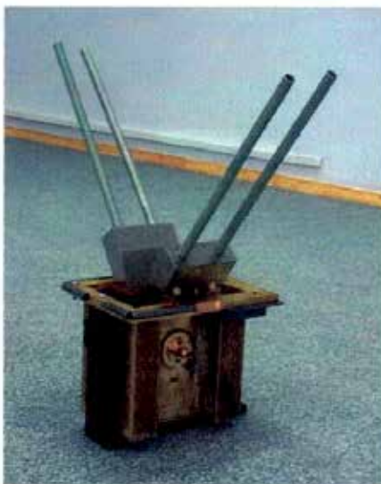
Fig. 2. Plasma dielectric antenna with four jet [8].
