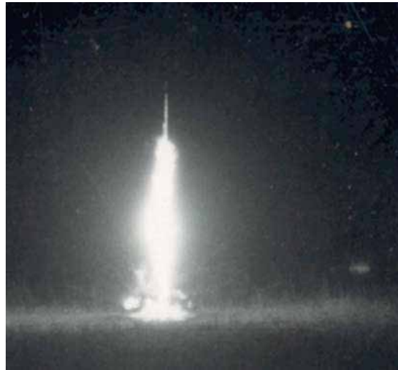
Fig. 17. Plasma dielectric antenna based on shaped charge with cylindrical liner.
