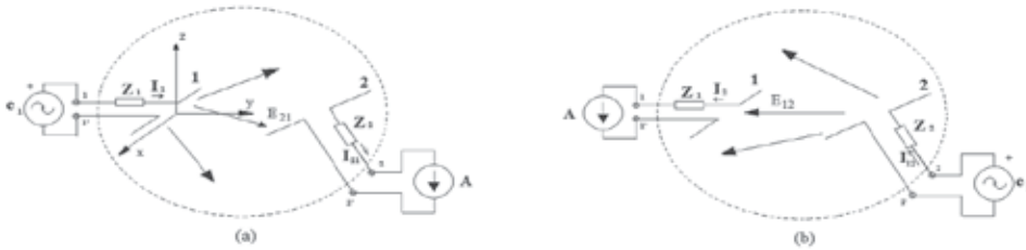
Fig. 2. Equivalent quadripole, linear and reciprocal, to study the interaction between a transmitter and a receiver antenna
