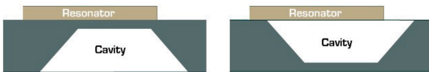
Fig. 14. FBAR processes: (a) Substrate etching (b) Substrate micro-machining.
