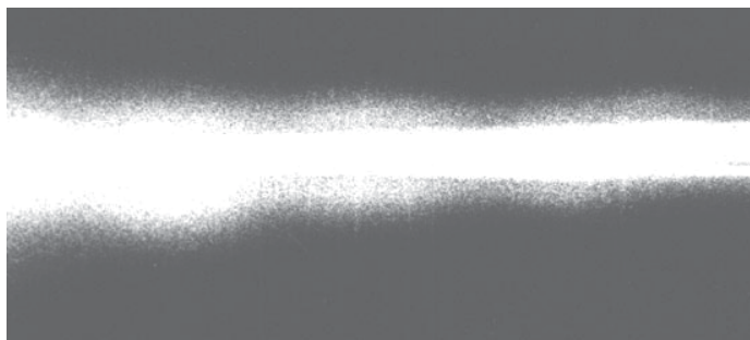
Fig. 13. Fragment of the plasma antenna shown the impulse character of the surface particle erosion.
