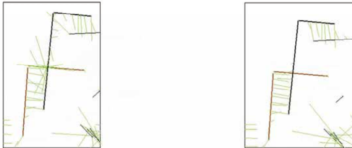
Figure 6. Left: forces between two scans (red lines belong to first scan, black lines to second scan) computed without direction information. Right: forces computed using L and K as described in example 2 (using equal masses). Correspondences between non parallel structures are weakened
