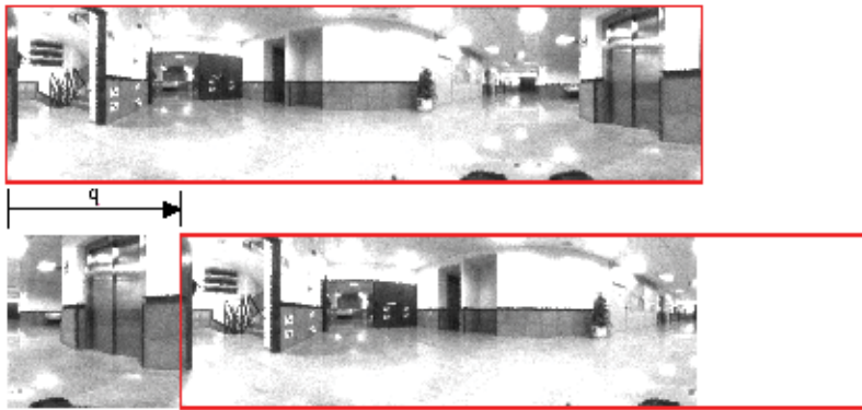
Figure 6. Two panoramic images taken in the same point but with different heading for the robot
