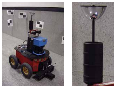
Figure 1. Pionner P3-AT robot and Catadioptric system that provides omnidirectional images
