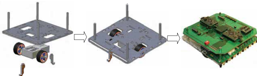
Figure 10. Mechanics of the behavioral control layer: CAD disassembled (left), CAD assembled (middle), completed mechatronics (right)
