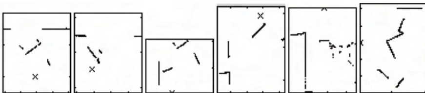
Figure 8. 6 out of 60 scans of the NIST rescue scenario data set. The scans in this data set are very sparse and have minimal overlap
