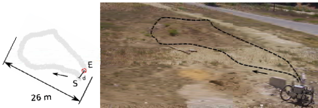
Fig. 8. A typical result of the visual-based dead-reckoning system. The estimated path on the left is superposed, with perspective correction, on a view of the terrain on the right. The superposing is illustrative only. The arrows represent the direction of motion, and the robot is on the starting position, represented by 'S' on the estimated path
