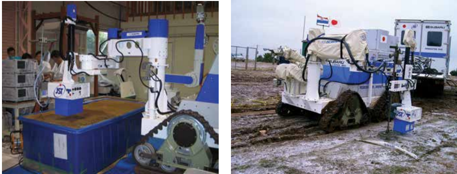
(a) SAR-GPR mounted on a robotic arm and scans in front of the MHV. (b) SAR-GPR in operation in CROMAC test site. SAR-GPR scans in the side of MHV
