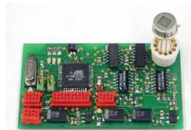
Fig. 1. The artificial nose sensor system. Left panel: schematic of each of the sensors of the 6 grid array including its main components. The size of a sensor is 0.18 \times 0.2 mm (with x length), with an active area of 0.032 mm 2 . Right panel: the full chemo-sensor package and its readout PCB. The sampling frequency of the PCB is 16.3 Hz, its dimensions 60 mm \times 35 mm, and its weight 13.8 g. Adapted from Pyk et al. (2006)
