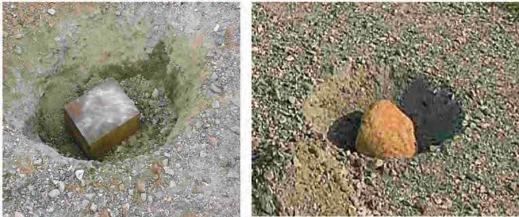
Fig. 19. Non-compliant false targets (steel block and stone) buried in gravel soil at depth 25 mm and 55 mm. Their nonlinear responses did not exceed the background level resulting in zero detection contrast
