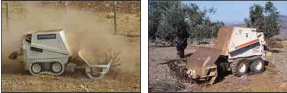
Fig. 2. The mini-flail vehicles “Božena 2 and 3”
