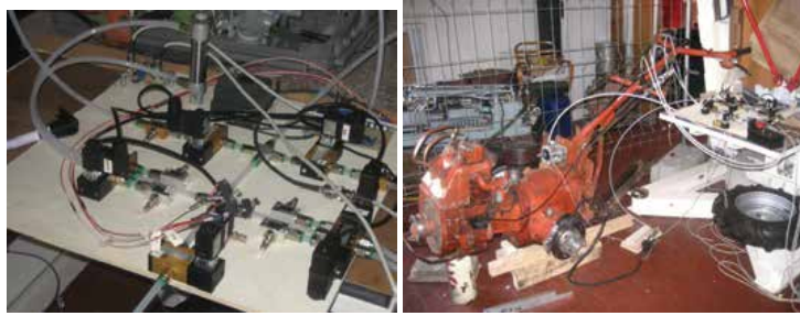
Fig. 13. Pictures of the valve bay and the control system assembled on the power tiller
