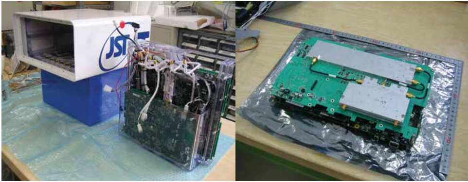
(a) Three vector network analyzers mounted in SAR-GPR
