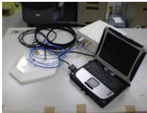
Fig. 4. Ground Penetrating Radar (GPR) system
