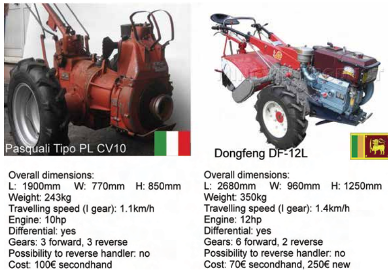
Fig. 4. Power tiller in use at the University of Genova Vs Power tiller available in Sri Lanka
