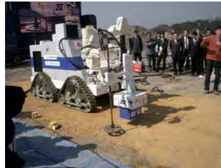
Fig. 8. Mine detection test of MHV
