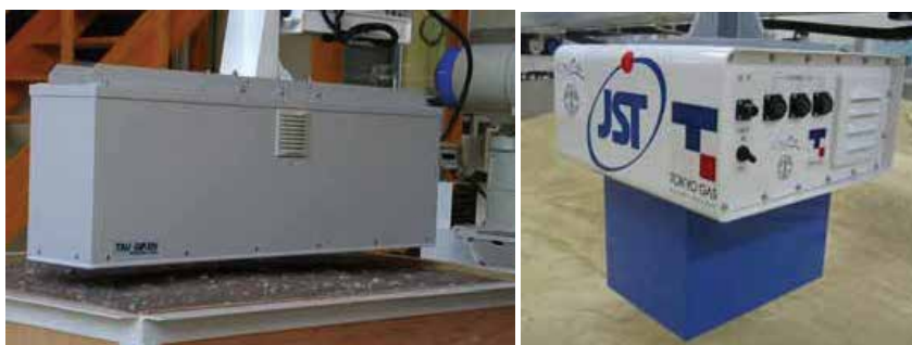
Fig. 31. Two interchangeable Radar sensor modules
