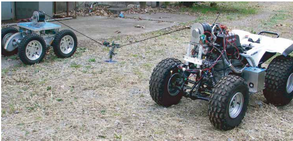
Fig. 2. Mine detection concept with hyper-tether and two mobile platforms
