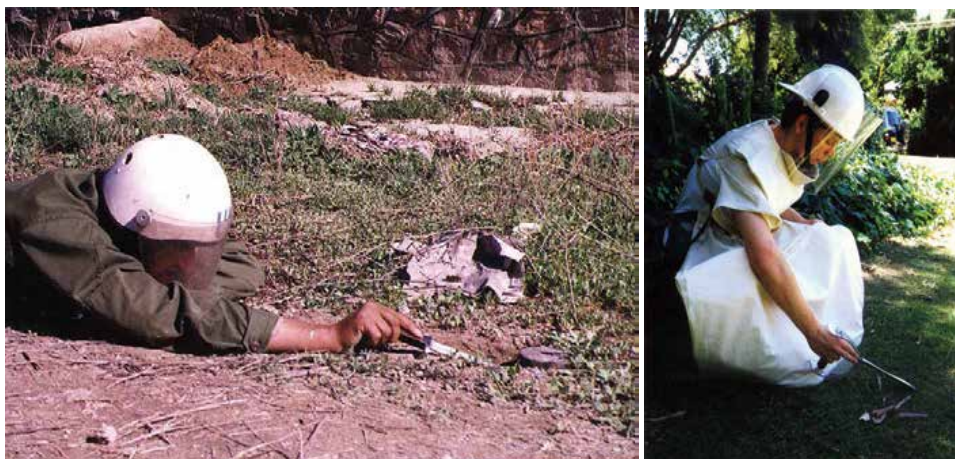
Fig. 1. Left: Prodding to investigate metal detector indication: Afghan deminers normally squat instead of the required prone position shown in this posed photo. Note the bayonet prodding tool and 1.5 kg military helmet with scratched visor. Right: Light weight helmet, visor, prodder with hand protection, and ballistic apron developed through research in Australia and Pakistan. The visor outer surface is protected by a replaceable scratch-resistant film. (photos: UN Mine Action Centre for Afghanistan, J. Trevelyan)
