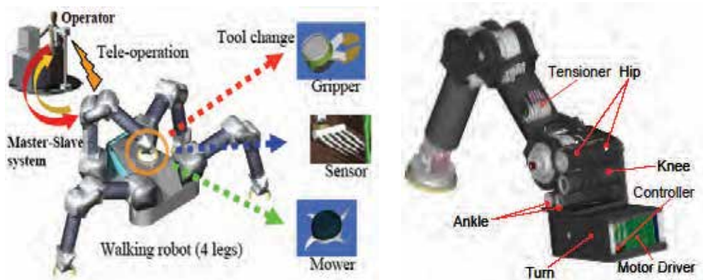
Fig. 27. The concept of TITAN-IX with implementation of the leg unit for the demining mission
