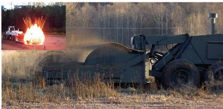
Fig. 3. Flail machine using hammers on the ends of spinning chains to clear vegetation and tripwires. This machine will also detonate a proportion of buried mines (inset). (photos: Scanjack AB, Sweden)
