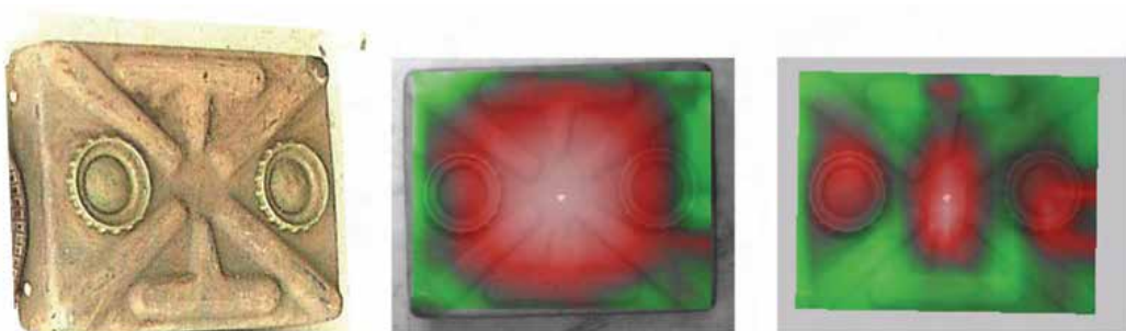
Fig. 5. Flexural modes of vibration of AT mine TMA-2 with the respective resonance frequencies 190 Hz and 490 Hz
