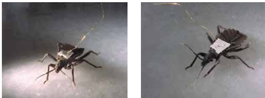
Fig. 9. Gold wire electrodes fixed on the back of an insect used to pick up electrical signals during the feeding process.
