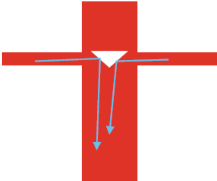
Figure 12. Basic scheme of a geometric rectifier. The horizontal arms of a dipole antenna intersect at the feed point. This feed point is shaped as an asymmetric defect that deflects charge carriers towards the bottom of the geometric rectifier [34].
