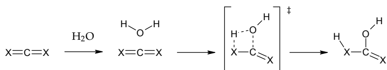
Fig. 8. Uncatalyzed reaction with water across a concerted four-membered cyclic transition state. \text{X} = \text{CH}_2, \text{NH}, \text{O}, \text{S}
