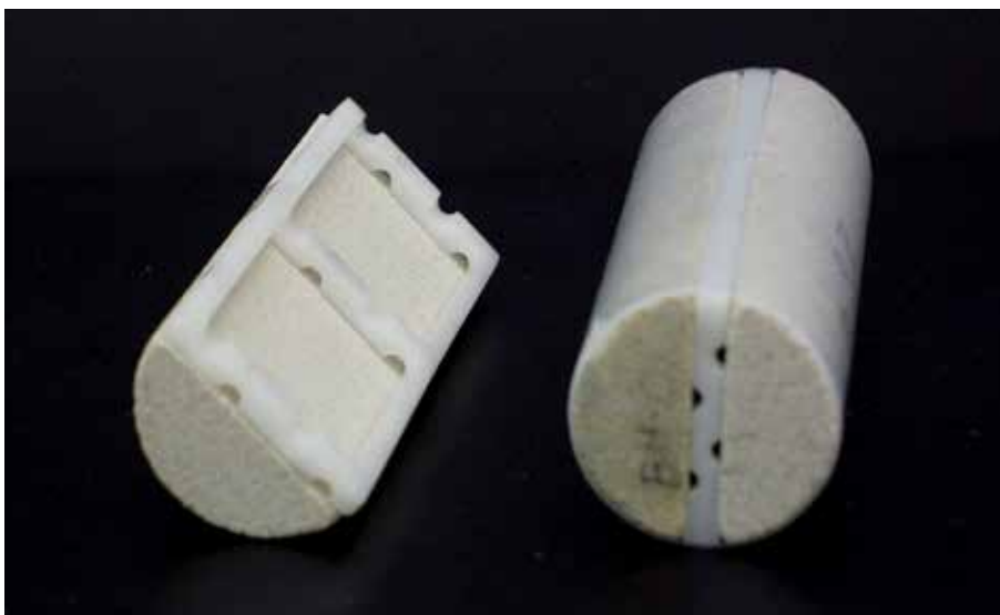
Fig. 8. Core design with spacer
