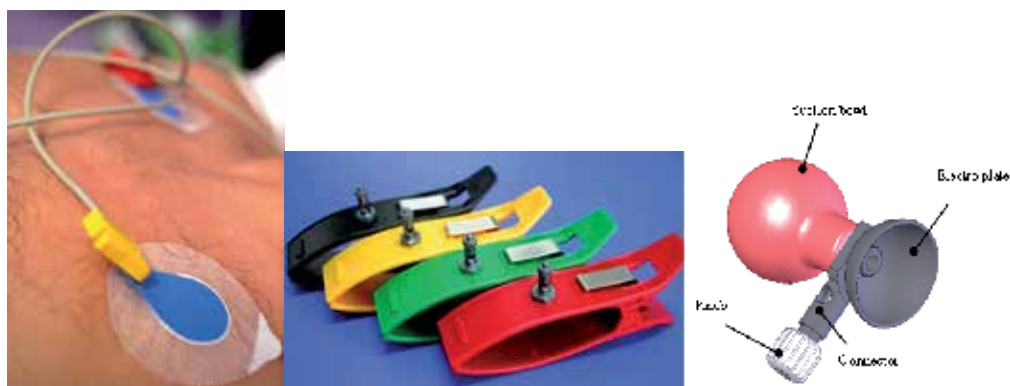
Fig. 2. Examples of ECG on-body electrodes commonly used for standard ECG: disposable, gel-impregnated, attachable electrodes (left), clamp reusable electrodes (center) and suction, reusable electrodes (right).
