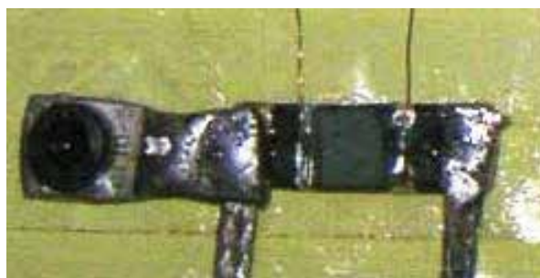
Fig. 7. Photograph of the system used to hold the Bi-2212 monoliths.
