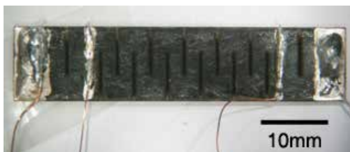
Fig. 16. Bi-2212 coating on a MgO substrate used for environmental degradation experiments with the sample immersed in water.
