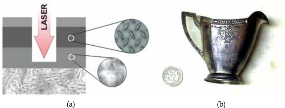
Fig. 7. (a) An schematic of in-depth laser microanalysis performed by LIBS technique, (b) The picture of Japanese Jug.
