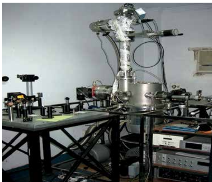
Fig. 9. Picture of our supersonic molecular beam linear time of flight mass spectrometer.
