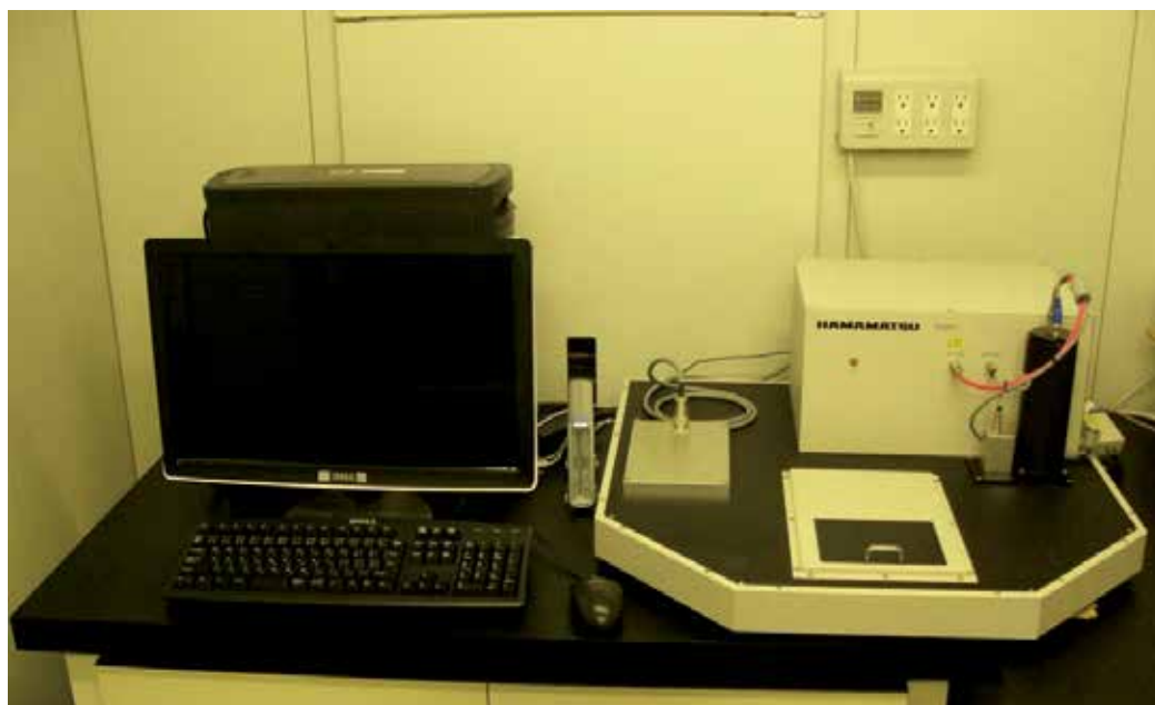
Figure 3. Appearance of photon counter CCSPC-01
