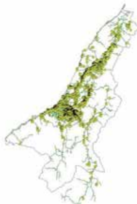
Figure 7. The observed points of the damaged poles due to the Chuetsu-Oki earthquake (treated as DI in Fig.4)
