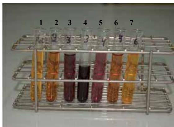
Figure 6. Cromazurol S Reaction 1.-Trideionized water pH=1.0 2.- K_2CrO_4 (50 \mu\text{g}/\text{mL} ) 3.- Cr(NO_3)_3 \cdot 9H_2O . (50 \mu\text{g}/\text{mL} ) 4.- Cr(NO_3)_3 \cdot 9H_2O . (500 \mu\text{g}/\text{mL} ) 5.- Problem (50 \mu\text{g}/\text{mL} ) 6.- Vitamin C (50 \mu\text{g}/\text{mL} ) 7.- Al_2(SO_4)_3 (50 \mu\text{g}/\text{mL} )
