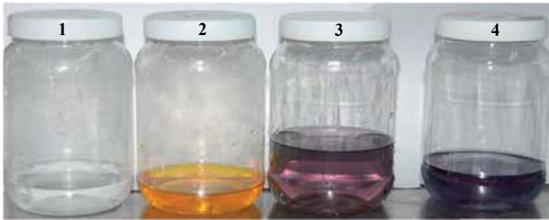
Figure 12. Chromium (VI) Reduction by lactic acid. 1. - Lactic acid standard solution (85%) 2. - Chromium (VI) standard solution (1.0 g /L). pH= 1.0 3.-100 mg Cr (VI)/L with lactic acid (100 mL) 4. - 1000 mg Cr (VI)/L with lactic acid (100 mL)
