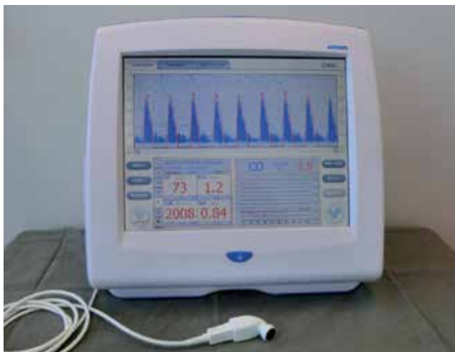
Figure 9. USCOM monitor showing Doppler signal data on its screen. The flow profiles are automatically outlined to measure stroke volumes. Below numerical readings are displayed. Lower right is a trend plot of saved cardiac output readings. The hand held USCOM probe is shown in front of the monitor. Ultrasound gel is applied to the probe to improve its acoustic contact.
