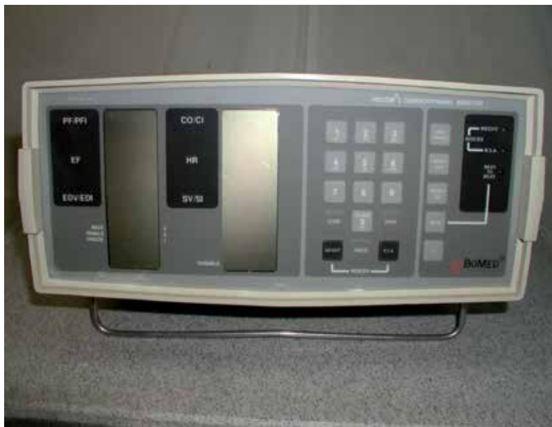
Figure 1. The BoMed NCCOM3. It connects to the patients using eight skin surface electrodes applied to the mid-neck and lower chest at the level of the diaphragm. Two additional ECG electrodes can be added. The BoMed is calibrated by inputting the patient's height and weight. Cardiac output and related bioimpedance variables are displayed as numbers. Data is averaged over 16 heart-beats.
