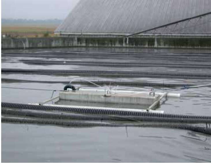
Figure 2. IRDA sampling device on a manure storage tank
