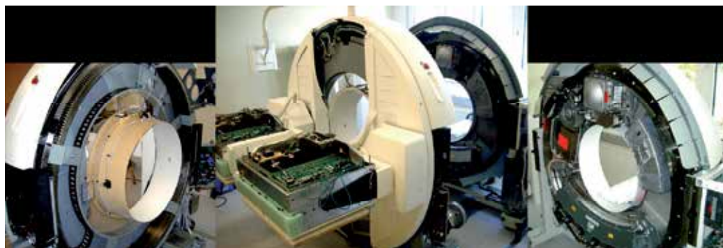
Fig. 3. Siemens Symbia T6: Left: Gantry of the dual head gamma camera, Center: both parts separated during service, Right: Gantry of the 6 slice MD CT
