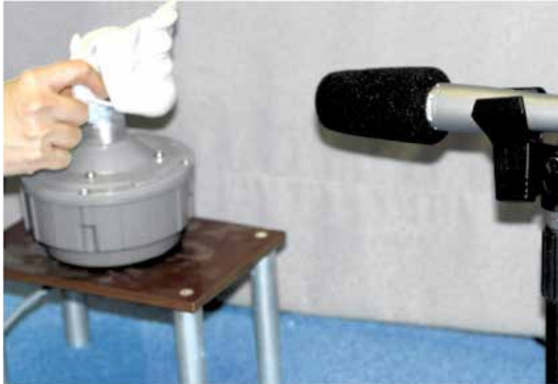
Fig. 13. Examination of analysis of vocal tract transmission characteristics using a model that was rapid-prototyped by our proposed method.
