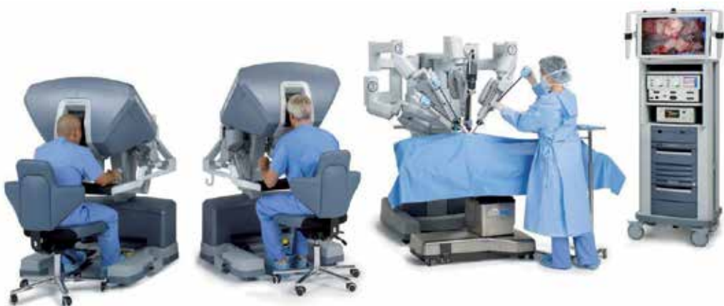
Figure 2. [26] : showing robotic and vision carts and the surgeon's console with an additional teaching console
