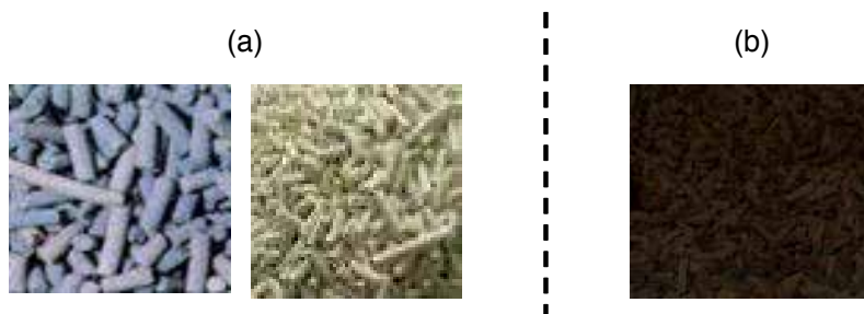
Figure 4. Typical hydrotreating catalysts (a) before use and (b) after use
