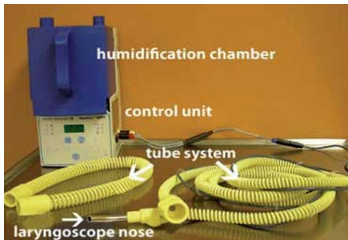
Figure 15. Device for moistening and warming-up of the respiration gas. The central unit (white) incorporates the electrical control unit. The humidifying chamber (blue) for single or multiple use is fixed at the central unit. The tubing system (yellow) is split into a short tube which transports the ventilation gas coming from the respirator to the humidifying chamber, and in a long tube which transports the now moistened and warmed-up gas from the humidifier chamber to the jet laryngoscope. The distal part of the long tube is metallic and is connected to the jet laryngoscope.
