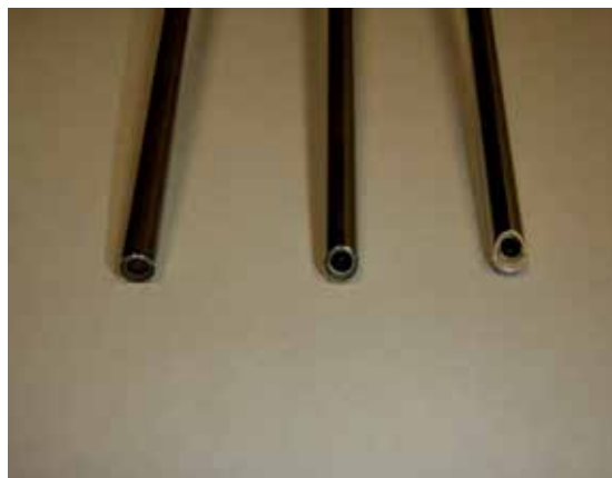
Figure 1. Telescopes, from left to right, 0, 30, 70 degree respectively.
