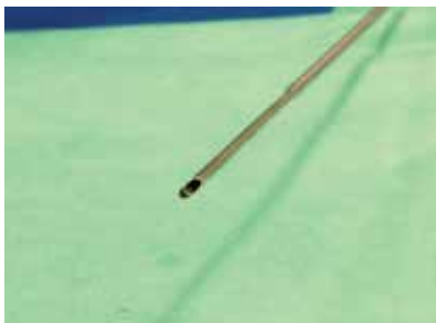
Figure 2. Distal tip of a semi-rigid ureteroscope showing the larger opening of the working channels (right side) compared to the optical opening. Note the stepped appearance as opposed to a more usually seen tapered tapered appearance. The lens is angled at 5 degrees to allow visualisation of the working instruments as they exit the channel.
