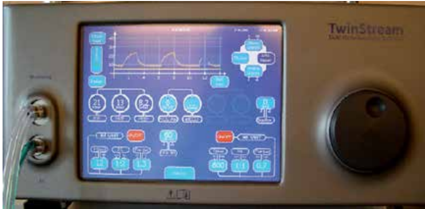
Figure 11. Jet respirator for the combined high-frequent and low-frequent jet ventilation (Twin Stream™ multimode respirator, Carl Reiner Ltd. Company with limited liability, Vienna, Austria). The continuous airway pressure is displayed in the left upper corner. The top right part shows the adjustable pressure limitation. In the middle left the digital airway pressure and in the center of the display the inspiratory oxygen concentration is displayed. On the lower left side the low-frequency jet unit can be seen and on the right there is the high-frequency jet unit.
