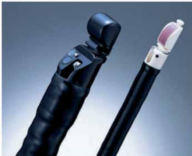
Figure 5. Devices used in endoscopic and endobronchial ultrasound. Endoscopic ultrasound probe (left) and endobronchial ultrasound scope (right) [105].
