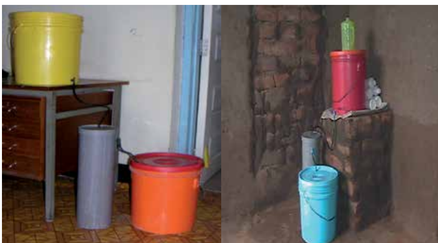
Figure 12. Household defluoridation unit employing bone char developed by Ngurdoto Research Station shown in average and low income household settings
