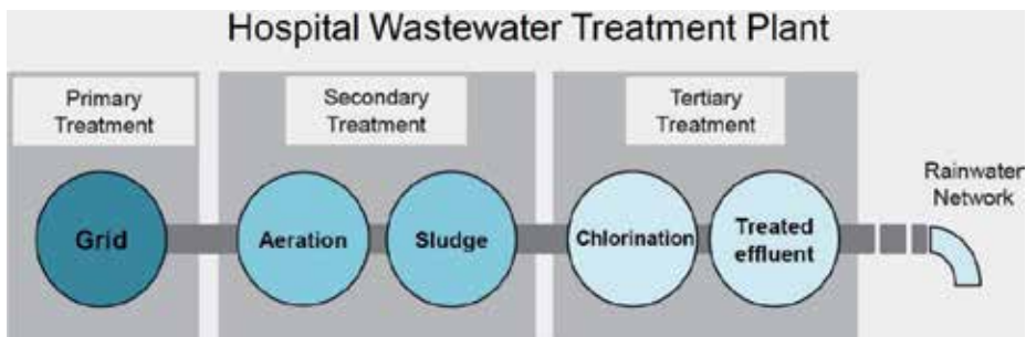
Figure 5. Schematic representation of the hospital's wastewater treatment plant.
