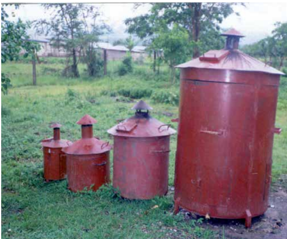
Figure 14. Different sizes of bone charring kilns as developed at the Ngurdoto Defluoridation Research Station
