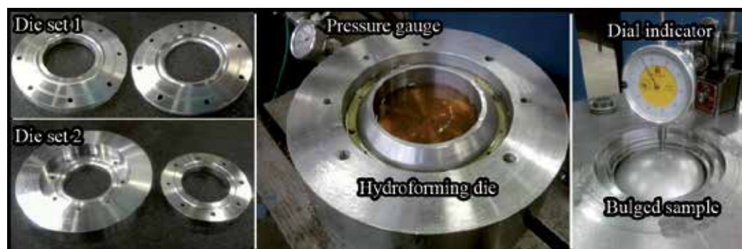
Figure 3. Hydroforming bulge test apparatus
