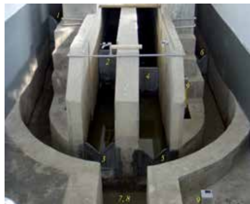
Figure 9. Discharge measurement structures for different runoff components from troughs with its location showing in Figure 8(a). 1- for rainfall; 2 and 3- for surface runoff; 4 and 5 – for interflow (30 cm below the soil surface); 6 – for interflow and groundwater flow (down to bedrock); 7 and 8 for total runoff (weirs are not shown). 1,3,5,6 and 8 are V-notch sharp-crested weir; 2, 4 and 7 are the full width rectangular sharp-crested weir; 9 is the tracking water head gauge. The picture design is the original concept, through renovations are now underway for gauge modernization.
