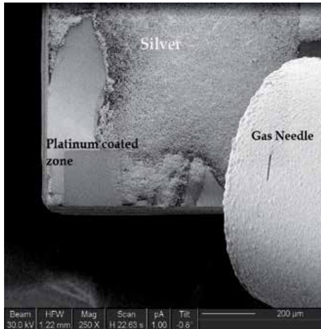
Figure 8. Secondary electron image of the sample with a square of Platinum coated zone made with gas deposition technique, the gas needle is also visible on the right hand of the picture.
