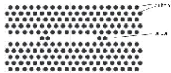
Figure 18. Schematic of L6 cavity to generate Raman effect.
