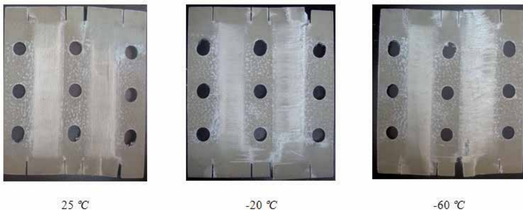
Figure 14. Tested specimens under shear loading at different temperatures
