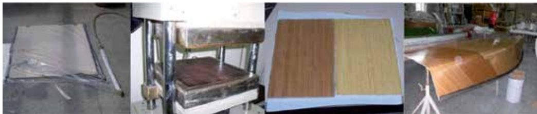
Figure 9. Manufacturing process of bamboo boat hull for water sports activities [40].
