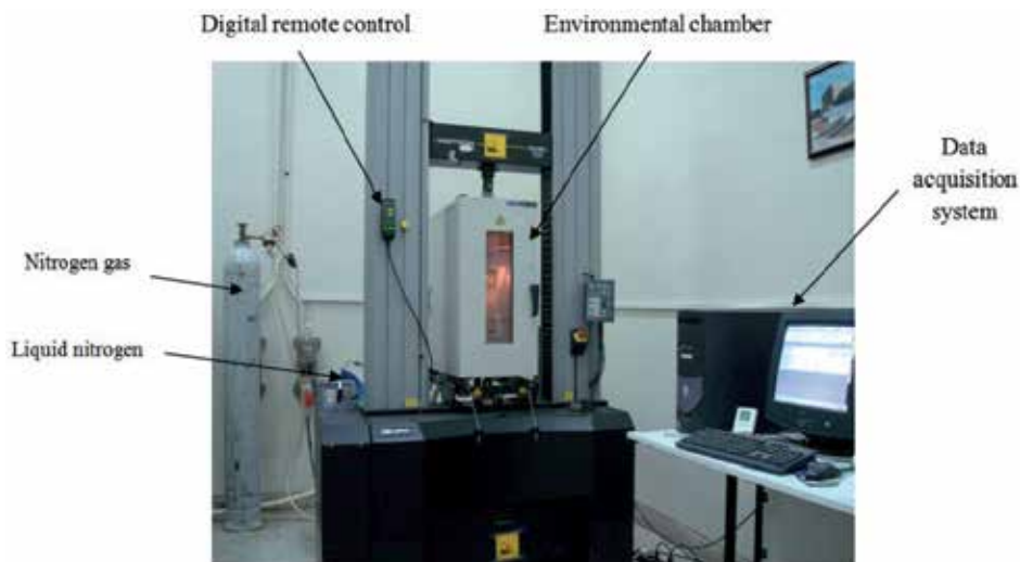
Figure 1. Experimental setup for mechanical tests at both room and low temperatures
