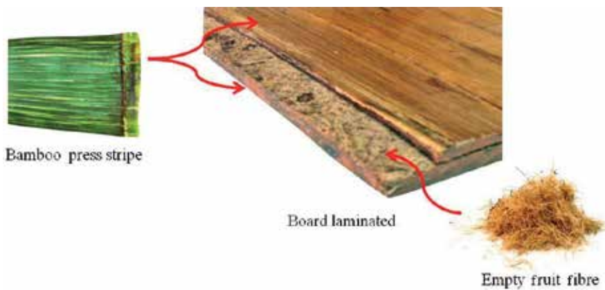
Figure 5. Crushed bamboo stripes laminated with empty fruit fiber.
