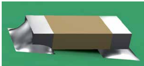
Figure 5. Reflection pattern on meniscus model with white ring illumination
