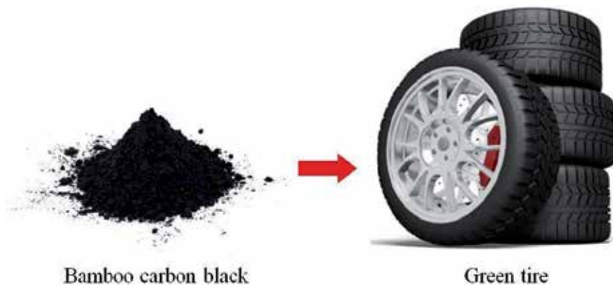
Figure 10. Green tire made from bamboo carbon black.
