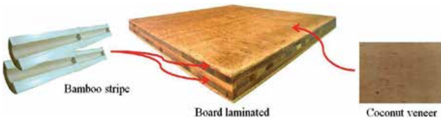
Figure 7. Coconut veneer laminated with bamboo stripe.
