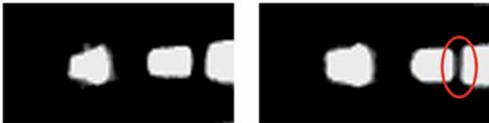
Figure 25. An example for the tiny differences between the images containing correct and faulty components
