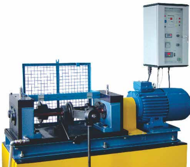
Fig. 17. T-12U Universal Back-to-back Gear Test Rig
