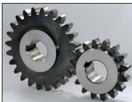
Fig. 15. Coated test gears used for testing pitting – type C-PT
