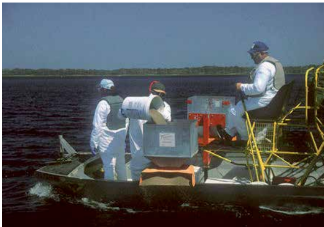
Figure 17. Application of granular herbicide using a boat-mounted spreader. Photo courtesy UF/IFAS Center for Aquatic and Invasive Plants.
