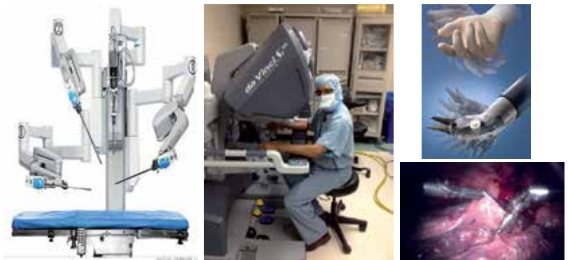
Figure 3. Robotic approach to lung resection is the latest evolution in lung resection. The surgeon operates from a remote location using the console to control the robot that is 'docked' to the patient. The instrument articulations are such, it is more versatile than the human hand, allowing detail dissection in small spaces, however lacks the tactile sensation.
