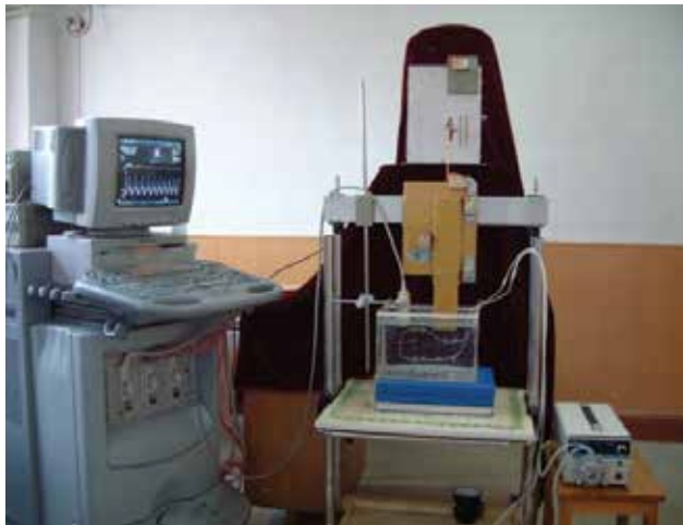
Fig. 1a. Photo of the whole set of the in vitro model experiment. From the right to the left of the photo the whole set is displayed. Right: the perfusion pump which drives the simulated blood in the tubing; Middle (from top to the bottom): the top is the TD-4 cardiac motion simulator (specially designed and home-made) that moves the plastic board up and down; the middle is the gears and connectors that connects the plastic board below; the bottom is the water tank with the plastic board in it. The tubing with 5% fiber-water slurry, the simulated blood, is fixed on the plastic board that is connected with the connector above. The plastic board with the tubing may move up and down freely by the simulator. The echo transducer is separately fixed on the frame of the setup; Left: Ultrasound machine, Sequoia 256
