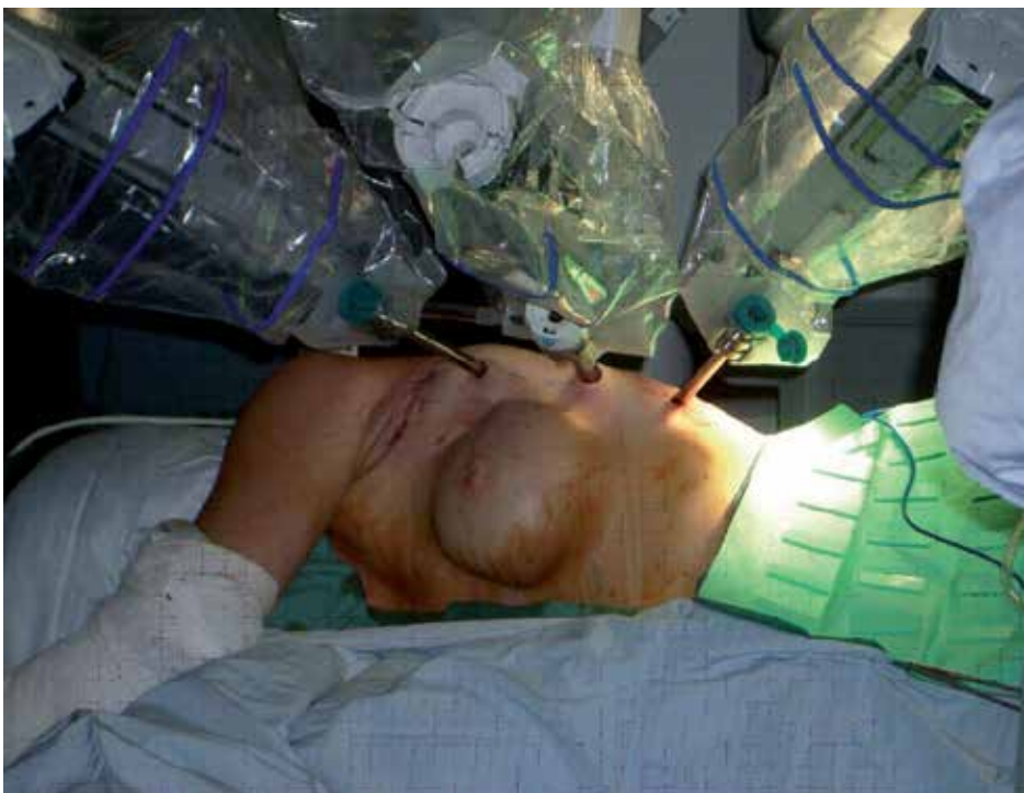
Figure 3. The robot is docked with the Patient-Side Cart behind the patient and the arms nearly parallel with the floor.
