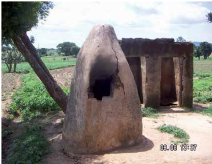
Figure 3. Locally developed incinerator using mud blocks
