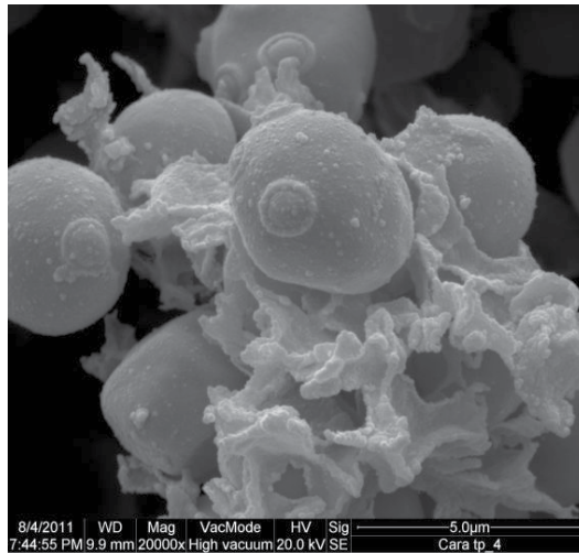
Figure 8. Scanning electron micrographs at magnifications of 20,000x Agar-agar and yam ( Dioscorea sp.) microspheres containing Saccharomyces cerevisiae Laboratory of Electron Microscopy and Microanalyses – State University of Londrina.
