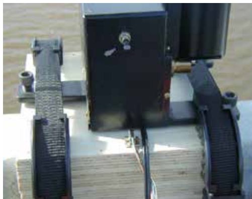
Figure 28. View of accelerometer fixed on wood support
