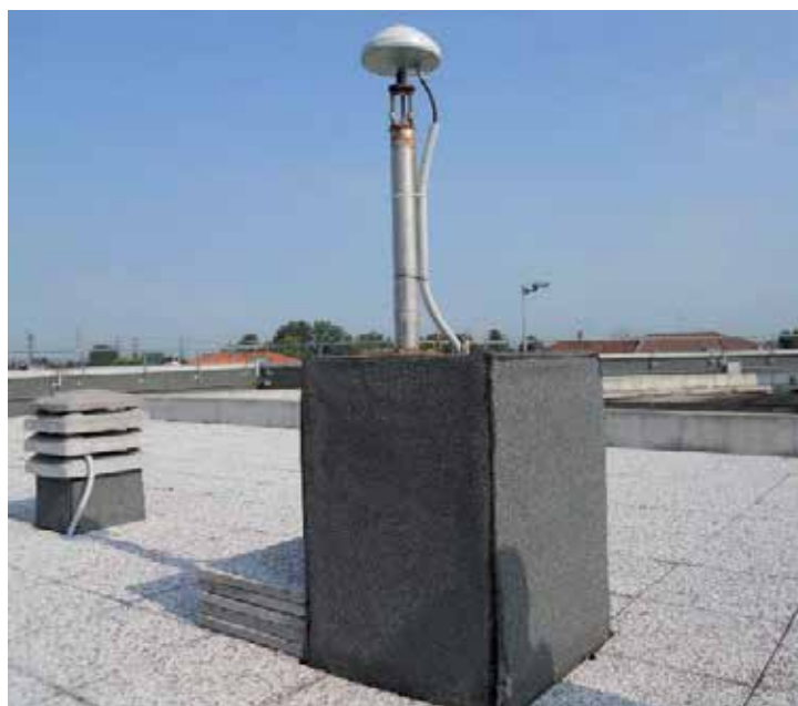
Figure 6. Pillar and antenna used for the NRTK test (VERC station)
