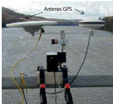
Figure 27. Wood support for electro-mechanical device
