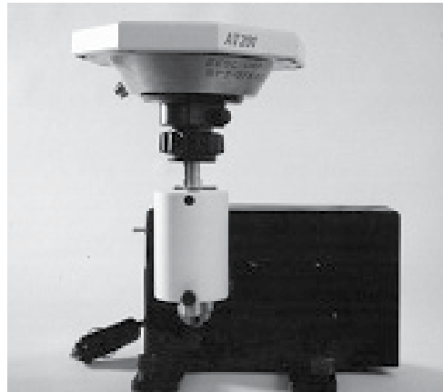
Figure 7. GPS antenna over the electro-mechanical oscillator
