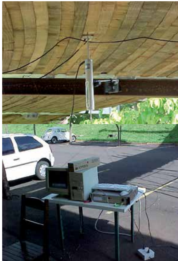
Figure 14. Transducer of displacements and data acquisition system
