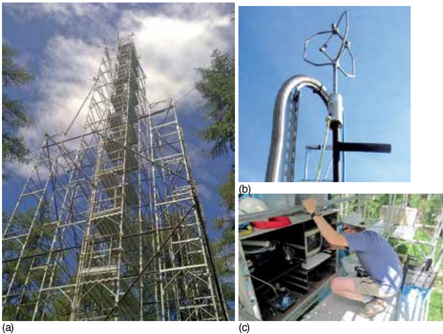
Figure 2. a) The flux tower in Paspardo; b) photo of the instrumentation installed on the top of the tower: the ultrasonic anemometer, the fast hygrometer and the inlet of the fast ozone analyzer; c) box at the bottom of the tower, inside the box there was the data acquisition system and the ozone reference analyzer
