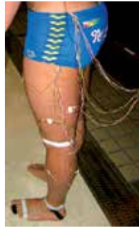
Figure 2. Electrodes and its codes attachment for underwater EMG experiment. [Picture was taken by the authors]
