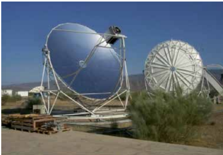
Figure 2. General description of Stirling EuroDish system [12]
