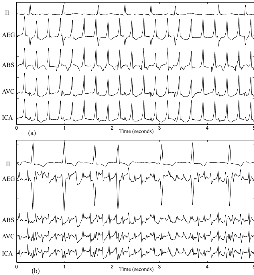
Figure 6. (a) From top to bottom, Lead II of an organized AF ECG shown for reference, the corresponding epicardial atrial electrogram (AEG), result of ventricular reduction with average beat subtraction (ABS), adaptive ventricular cancellation (AVC) and independent component analysis (ICA). (b) This panel plots the same information as panel (a) for a disorganized AF ECG. Note how ABS does not distort the resulting signal in this latter case [31].
