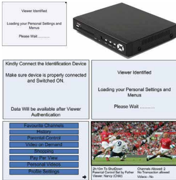
Fig. 6. (a) IPTV Viewers Identification Screen Capture (b) Experimental Platform with Screen Capture and Display.
