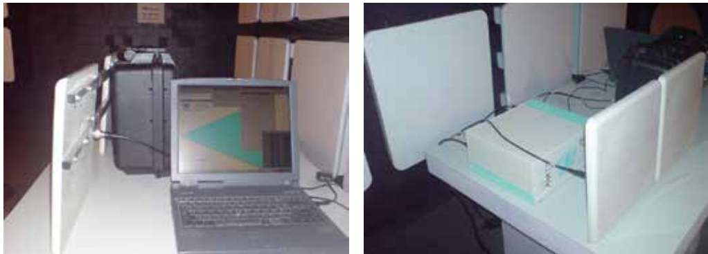
Fig. 1. The RFID system on the turn-table in the anechoic chamber with the control computer connected to the Ethernet network via optical-fibre isolated converters
