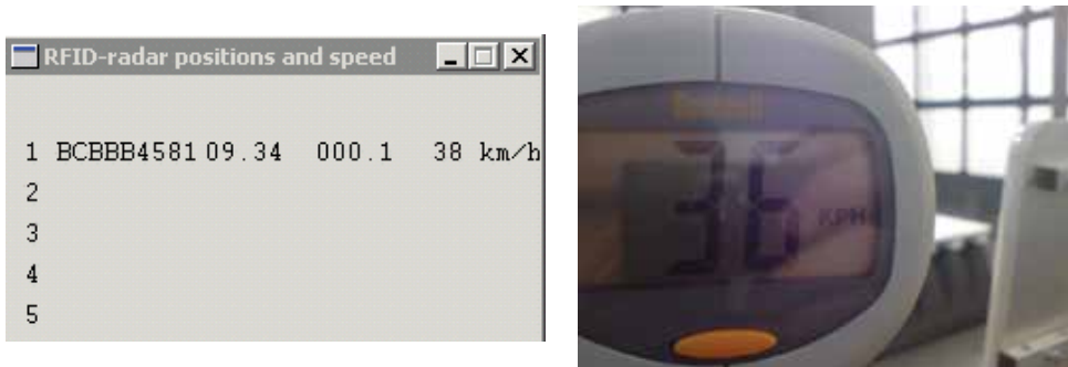
Fig. 17. Comparison between the speeds measured by the RFID system and a K-band radar
