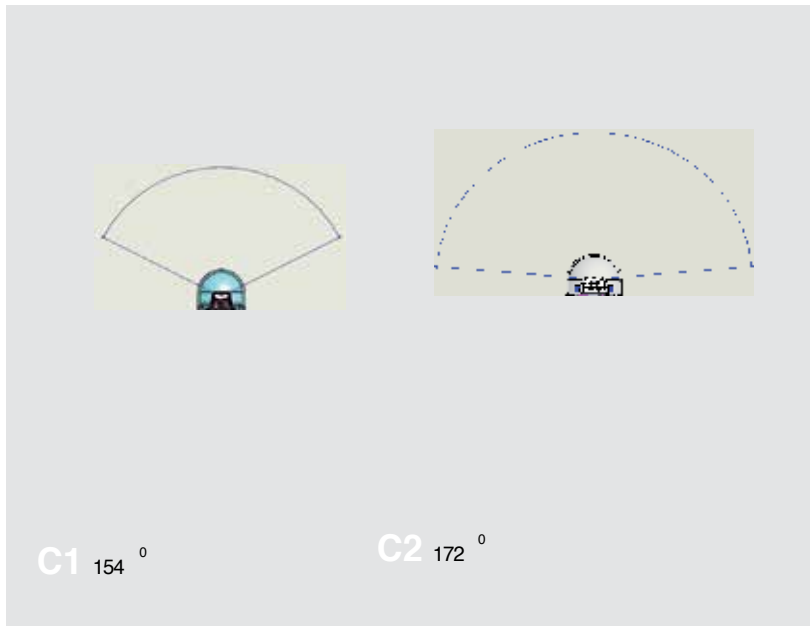
Figure 2. The left side image demonstrates the angle of view of the out dated C1 colon capsule. The right hand image demonstrates the angle of view of the C2 colon capsule with a near panoramic view.
