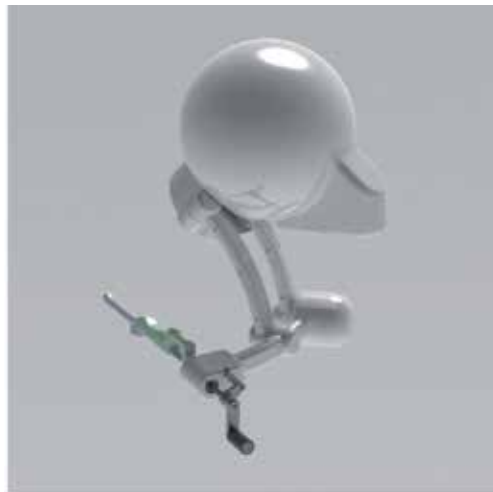
Figure 8. A schematic diagram of the mechanical tracker, which supports the TRUS transducer and attached cradle. This configuration constrains the TRUS probe motion to three degrees-of-freedom and one degree of translation along the axis of the probe. The system is mounted at the base of a stabilizer while the linkage allows the TRUS transducer to be manually manipulated about a remote center of motion (RCM), which is at the center of the ultrasound transducer tip.
