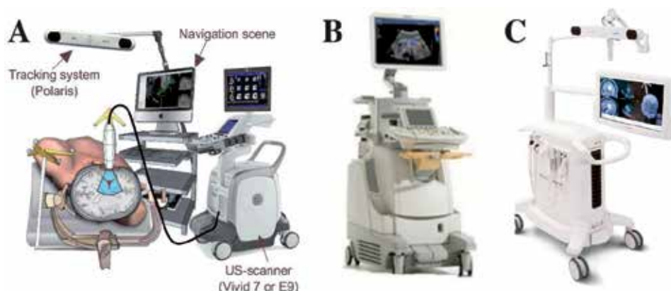
Figure 13. Different approaches to integrating (3D) ultrasound and navigation. A) A two-rack solution and examples of one-rack solutions (B and C).
