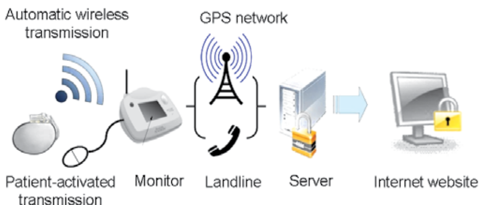
Fig. 1. Components of remote monitoring system. Systems differ regarding data transfer, which may require patient's active involvement or is performed wirelessly from the implanted device to a patient monitor. Data from the patient monitor is sent to a central database using either an analogue phone landline or via GSM network. The data are accessible to the clinical staff on a secure Internet site.
