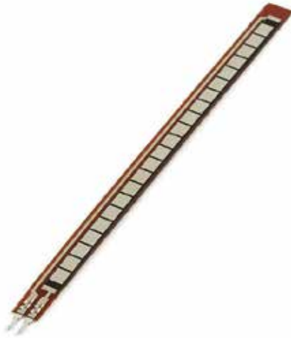
Fig. 6. The flex sensor: the sensor used to measure a knee movement variable in our proposed system. Image from: www.sparkfun.com
