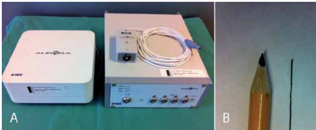
Figure 2. A) Electromagnetic tracking system - NDI Aurora. (B) Tracking sensor – 0.5 mm diameter
