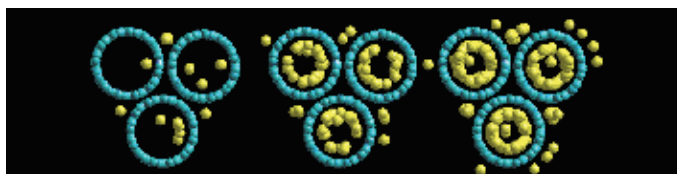
Fig. 12. Upper view of filling evolution corresponding to isotherm at 113 K and pressures of 1.38, 6.27, 56.3 Pa for opened end tubes of 1.628 nm, (12,12) SWNT. (Adapted from Albesa et al., 2010) Copyright 2010 American Chemical Society
