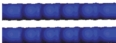
Fig. 16. The distribution of the electron charge for undamaged bilayer graphene (the density equals 0.4 \text{ el} / \text{A}^3 ).
