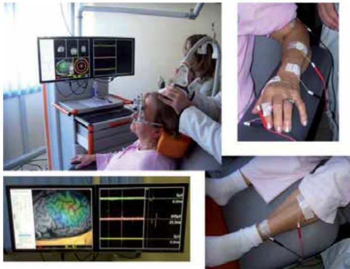
Figure 1. The navigated brain stimulation system Nexstim (Nexstim Ltd., Helsinki, Finland). With NBS, conventional transcranial magnetic stimulation is combined with a neuronavigation system that allows precise identification of each single “stimulated” point in the cortex on three-dimensional imaging study of the patient brain. Muscles responses to electric field (motor evoked potential, MEP) are recorded using EMG channels. The motor map obtained can be used for pre-surgical planning and integrated in the neuronavigation during surgical procedures.
